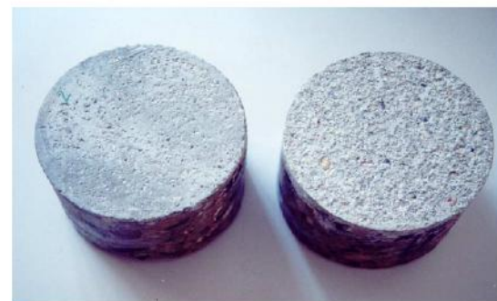
Figure 2: surface after the freeze - thaw tests in salty solution.
